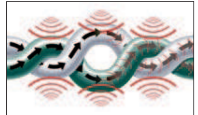
Illustration 1: Example of Non-Bonded-Pair. As cable is stretched and pulled, pairs begin to separate, causing a degradation in signal quality.
