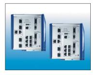
RSR series switches are available with optional gigabit ports and an extended temperature range of -40 °C to +85 °C. Ultra-fast ring recovery times under 10 ms are possible using HIPER-Ring redundancy protocol and the switch's robust metal housing offers extended RFI/EMI and vibration immunity.
