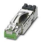
RJ45 connector, Degree of protection: IP20, Number of positions: 8, 1 Gbps, CAT5 (IEC 11801:2002), Material: Zinc die-cast, Connection method: IDC fast connection, Connection cross section: AWG 23-22, Cable exit: straight
