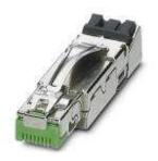
RJ45 connector, Degree of protection: IP20, Number of positions: 8, 1 Gbps, CAT5 (IEC 11801:2002), Material: Zinc die-cast, Connection method: IDC fast connection, Connection cross section: AWG 26-24, Cable exit: straight
