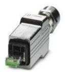
Push-pull connector (version 14), die-cast zinc, with RJ45 connector insert, 8-pos., with IDC fast connection technology, for 1 and 7-wire cores, 26 ... 24 AWG, for cable diameter of 5.5 mm ... 10 mm
