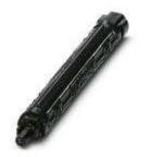
Fuse connector for protecting modules and devices in photovoltaic systems, black, SUNCLIX pin connector pattern, 1500 V/8 A, IP68 (24 h/2 m)
