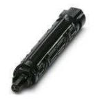
Fuse connector for protecting modules and devices in photovoltaic systems, black, SUNCLIX pin connector pattern, 1000 V/10 A, IP68 (24 h/2 m)
