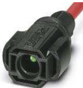
Photovoltaic connector, nominal current: 40 A, nom. voltage: 1500 V, connection method: Crimp, color: black. can only be released using a tool
