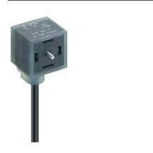
Actuator cordset, single-ended, valve connector according to DIN EN 175301-803, form A, with LED function indicator, varistor voltage protection, connected protective earth
