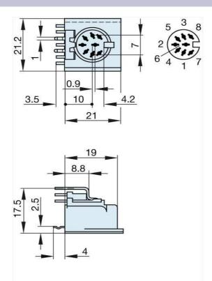
Arrangement of the soldering points on the components side
