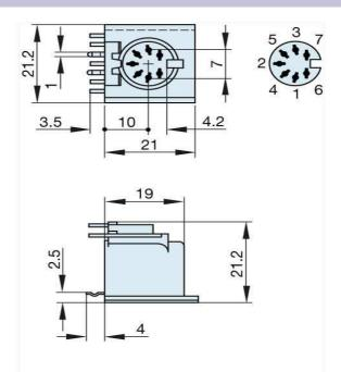
Arrangement of the soldering points on the components side
