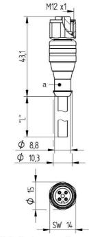
\*a Protective hose mounting Schutzschlauchmontage
