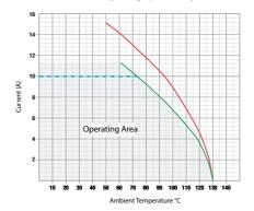
7000 Series Current vs. Temperature Characteristics
