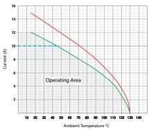
7000 Series Current vs. Temperature Characteristics 32 Pole, Plastic Body, Crimp Terminal, 22 AWG wire
