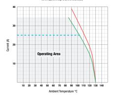
7000 Series Current vs. Temperature Characteristics
