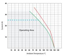
7000 Series Current vs. Temperature Characteristics
