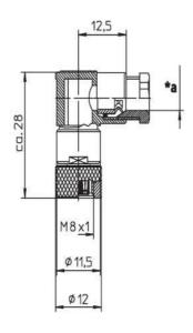
\*a Kabelverschraubung Screw joint for cable
