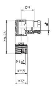
\*a Kabelverschraubung Screw joint for cable
