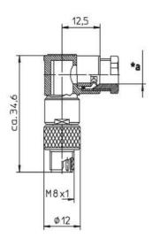
\*a Kabelverschraubung Screw joint for cable
