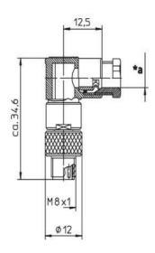
\*a Kabelverschraubung Screw joint for cable
