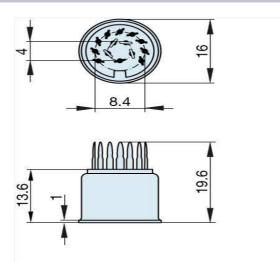
Arrangement of the soldering points on the components side
