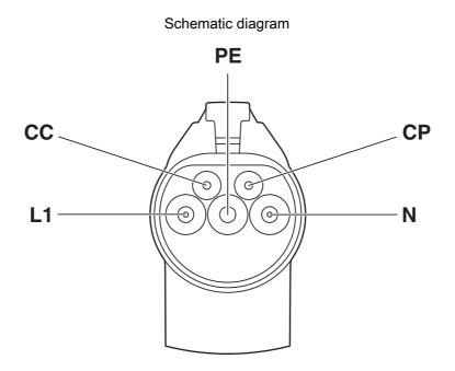
Pin assignment of the Vehicle Connector
