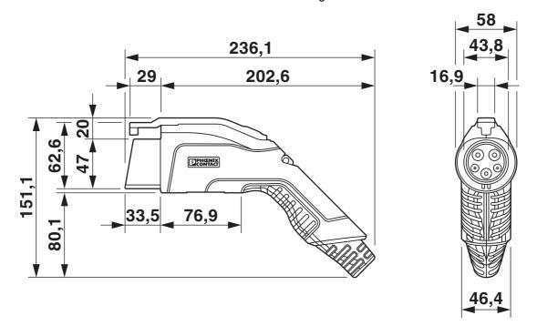
Make sure that the vehicle charging connector is placed in an appropriate charging connector holder, which ensures a minimum protection rating of IP24 in accordance with IEC 61851-1, for the entire time between charging. To create this charging connector holder, use the dimensions of the vehicle charging connector. Detailed dimensions can also be found in the Download area.
