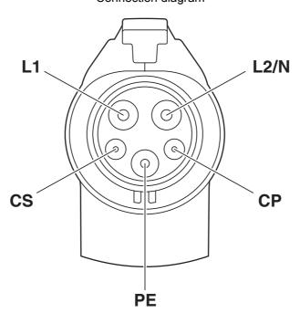
Pin assignment of the Vehicle Connector
