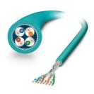
Data cable, Ethernet  $CAT6_A$  (10 Gbps), 8-position halogen-free, shielded, free cable end, on free cable end, cable length: Free entry (0.5 ... 400 m)
