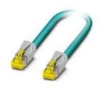
Patch cable,  $CAT6_A$ , 4-pair, shielded, connection not crossed (line), assembled at both ends with RJ45/IP20 connectors, outer sheath material: PUR, length: 3.0 m
