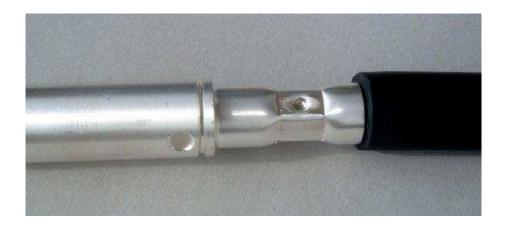
**5.** Examine the crimped joint to ensure that the crimp is satisfactory. Ensure that all of the conductor strands are contained within the crimped area.
