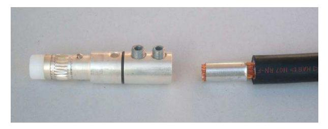
**4.** Select the appropriate reduction sleeves (see Table 1 below) and slide on in sequence over the exposed conductor stranding. All sleeves down to the size recommended for the cable in use should be used. i.e. for the 50m2 cable, the R120, R95, R70 and R50 sleeves should all be used. The sleeves fit inside each other to give a gradual reduction in diameter. The flared end of the sleeves should be against the cable insulation.
