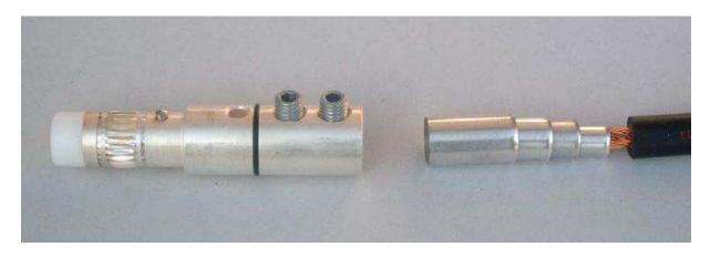
**5.** Slide the cable and reduction sleeves into the rear of the contact ensuring that they are fully seated inside of the contact. Using a 5mm A/F Allen key tighten the set screws to the appropriate torque setting.
