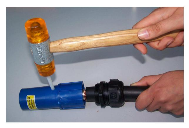
**9.** Screw the cable gland into the insulator, tightening to a torque of 13Nm minimum.
